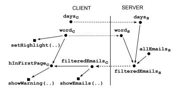
**Fig. 3.** Dependency graph among reactive values in the SimpleEmail application. Dashed arrows indicate over-network dependencies, square nodes indicate observers with side effects.
